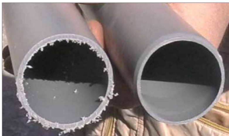
Tubo in plastica prima e dopo la sbavatura. Plastic pipe, before and after cleaned with our rimmers.
